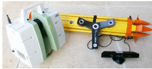
Figure 3: Three devices used for capturing the input data for our system. From left to right, a Leica ScanStation C10 static laser scanner, a FARO Freestyle X hand-held scanner, and a Microsoft Kinect One depth camera.
