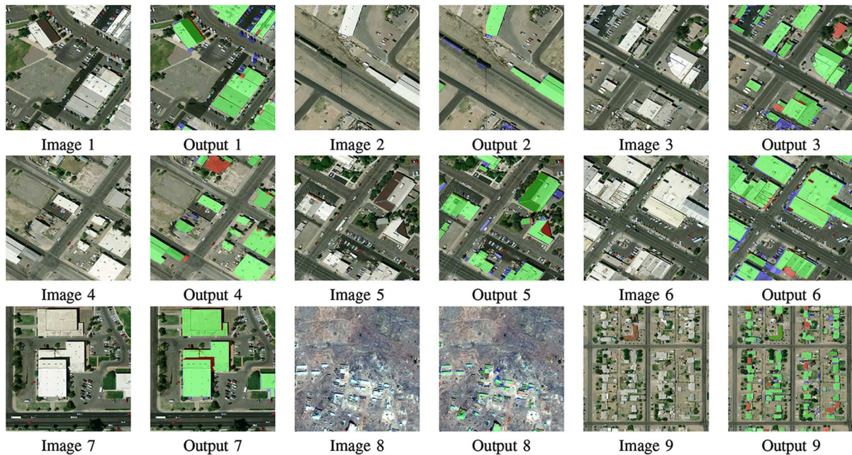
Fig. 16. (Odd column) test images #1–9; (even column) segmentation results for test images #1–9. True positives are tinted green, false negatives are tinted red, and false positives are tinted blue.
