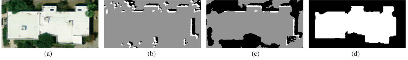
Fig. 4. Example of successful roof detection when the shadow has gaps (notice the trees obstructing the shadow of the building): (a) roof image; (b) initial foreground/background assignment; (c) foreground/background labels with additional vegetation constraint; and (d) result of grabcut on (c).
