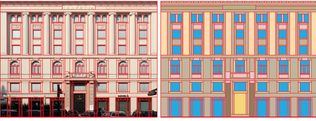
Figure 5: Left: a segmented facade image with region boundaries shown in red. Right: terminal-regions labeled according to their material.
