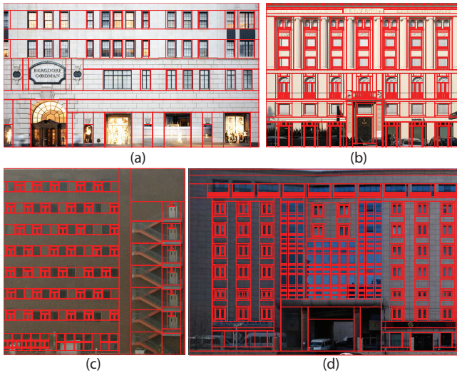
Figure 2: Facade examples that show instances where the model of Mueller et al. would lead to the splitting of facade elements. (a) has large elements in the first floor and smaller windows in the top floors. There is no meaningful grid structure. (b) The door spans two floors and the columns on the top span two floors. The columns themselves also create an interleaved grid of elements that cannot be modeled. (c) The irregular arrangements of the windows makes it impossible to find vertical splits that do not cut through a window. (d) The structure around the door and the fine glass paneling make splitting into tiles impossible.
