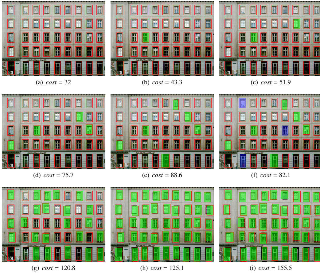
Figure 13: The grammar sizes of a facade layout with different types of random noise. (a) Input facade layout. (b) One rectangle is randomly moved horizontally (marked as the green rectangle). (c) Two rectangles are randomly moved horizontally. (d) More rectangles are randomly moved vertically and horizontally. (e) Both the rectangles' positions and sizes are randomly changed. (f) Rectangles are randomly deleted (see the blue rectangles). (g) Half of the rectangles are randomly moved. (h) All of the rectangles are randomly moved. (i) All of the rectangles' positions and sizes are changed.
