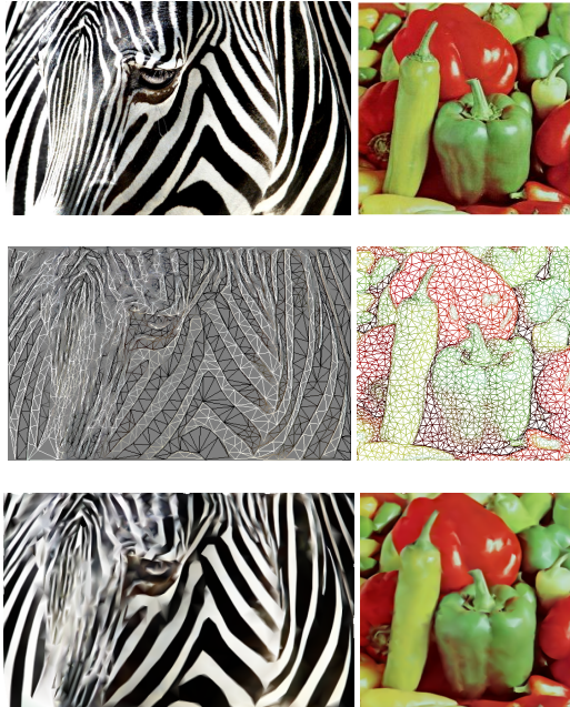
Figure 4: Top row is original images of Zebra and Bell peppers. Middle row is the base mesh and bottom row is the base mesh rendered with OpenGL shading resulting in images close to the original. The base meshes for the two images were created with an optimization for colour distortion to preserve the features, black and white stripes in the Zebra and pepper boundaries in the Bell peppers.
