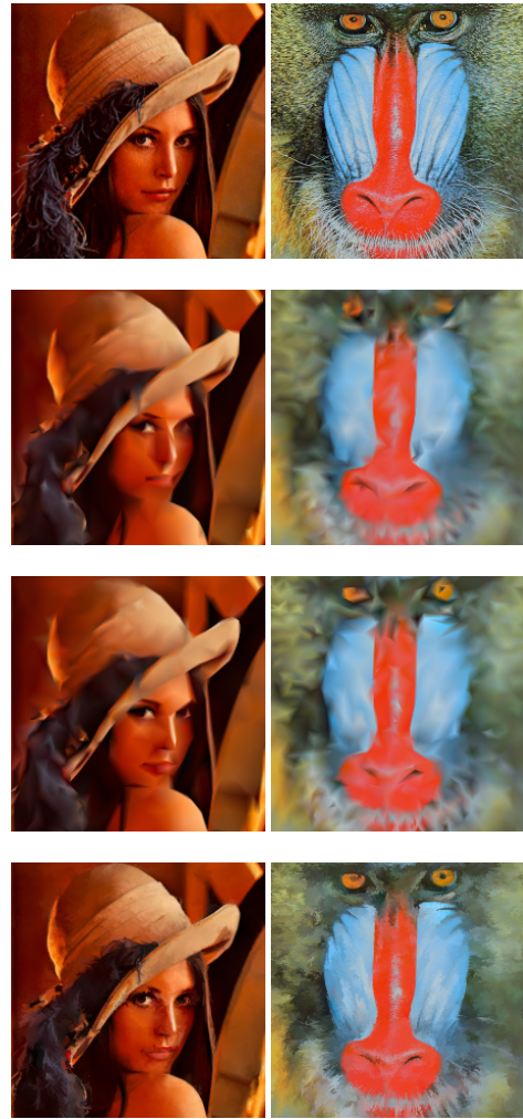
Figure 1: From top down: original images of Lena and Mandrill. Second and third rows represent base meshes using Hoppe's and our method respectively; base meshes have 1300(Lena) and 1960 (Mandrill) faces. The fourth row shows the reconstruction by interpolating the colour using our parameterization. There is no visible discontinuity across the base mesh faces. It qualitatively shows that our parameterization is globally continuous and has small distortion in the feature space.
