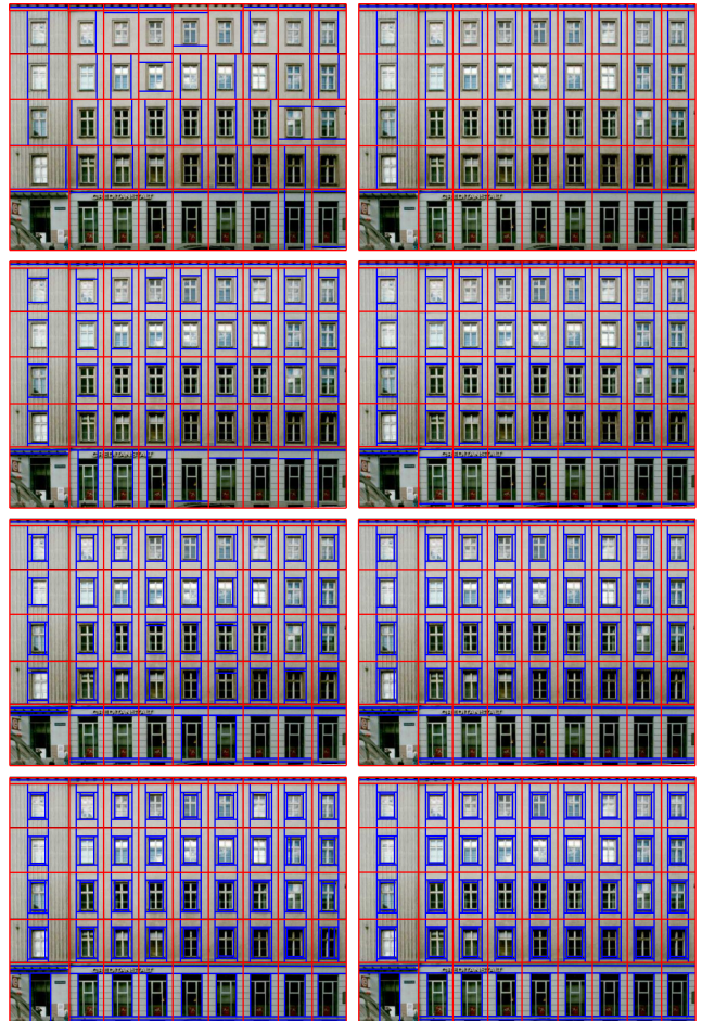
Figure 10: This derivation sequence illustrates the impact of the global split synchronization. Left: the algorithm without synchronization. Right: synchronization can eliminate almost all errors.
