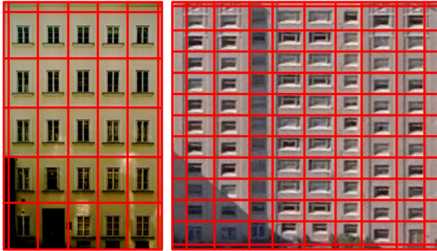
Figure 4: In the first stage of the process, the facade is automatically subdivided into tiles (illustrated as red lines). Moreover, similar tile appearances are detected and registered in groups.
