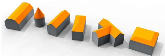
Figure 7: Selected roof types. From left to right: gambrel, cone, gabled, hipped, cross-gable, mansard.
