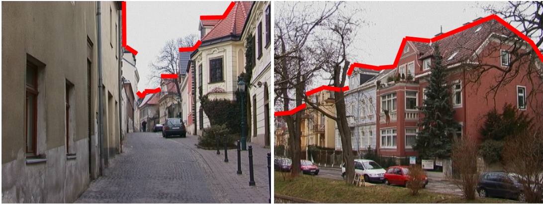
Figure 2.3: Occlusion in urban environments is essentially 2.5 dimensional. The occlusion of a building can be described by its roof edges, shown in red.
